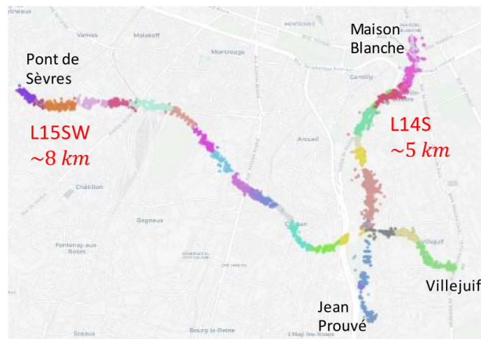
Figure 14 – View of the settlement sensors used in the analysis of the lines 14S and 15SW using ML (Richa et al, 2023)
